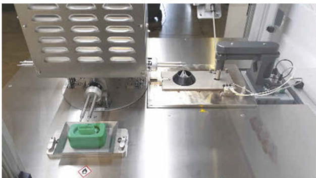
Fluxing and tinning position, easy accessible and exchangeable for cleaning and maintenance.
