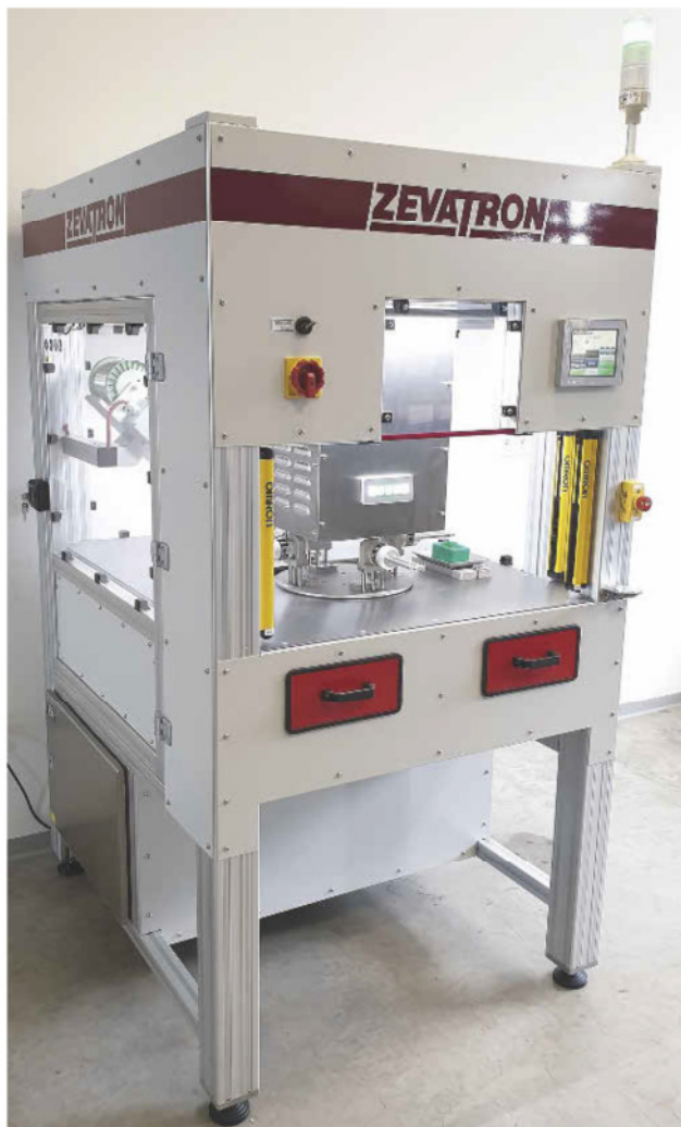
Rotary tinning station with 4 positions and encoded trays for nio parts.
