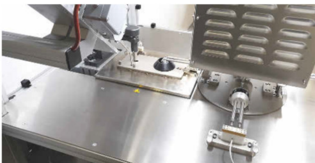
Solder pump system with customized nozzles, automatic solder supply, continuity test.
